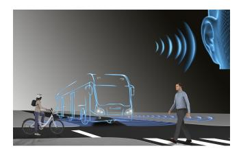
The AVAS is an acoustic warning system for hybrid and electric vehicles designed to increase the safety of road users. Once a pre-defined speed has been reached, the noise fades in / fades out. An acoustic signal is also automatically given off when reversing. The driver can easily activate or deactivate the warning system by means of a switch. The AVAS consists of a dustproof and waterproof housing.
